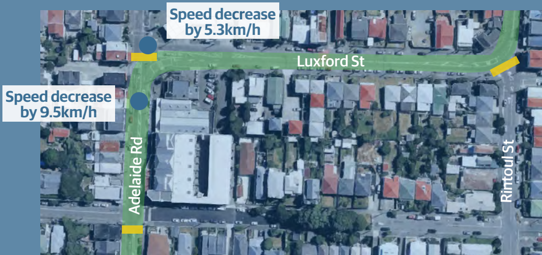
Figure 113: Traffic speed measuring - Luxford St and Adelaide Rd
