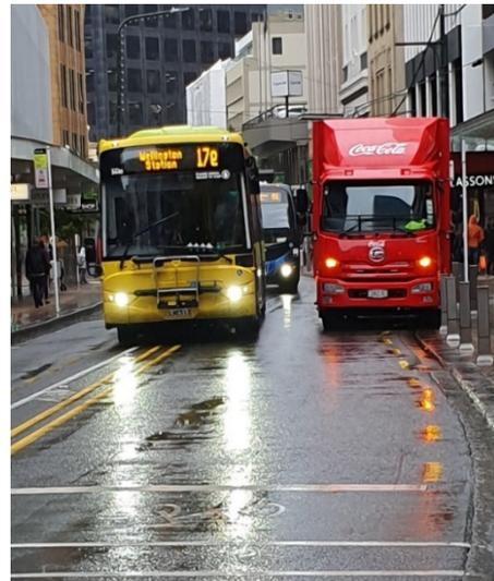
Delays associated with kerbside facilities are caused by their location and design. The red truck in Figure 17 is illegally parked opposite the Lambton Quay / Hunter Street Southbound bus stop. It shows northbound buses forced to cross the centre line. When southbound buses are waiting at the stop, northbound buses would be delayed.
