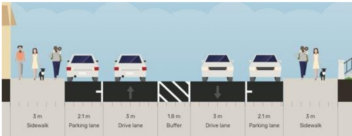
Figure 54: Karori Rd/SKR Segment 3 existing cross section
