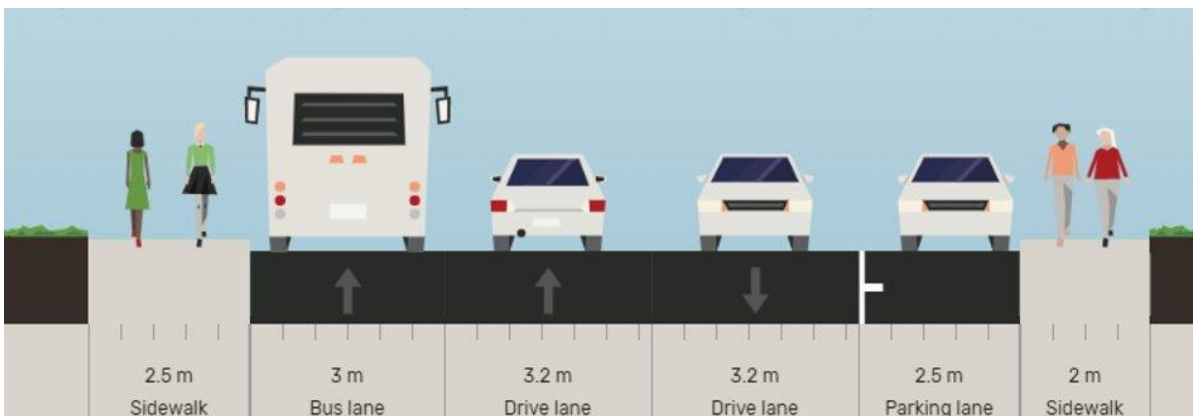
Figure 16: Glenmore St Segment 3 existing cross section
