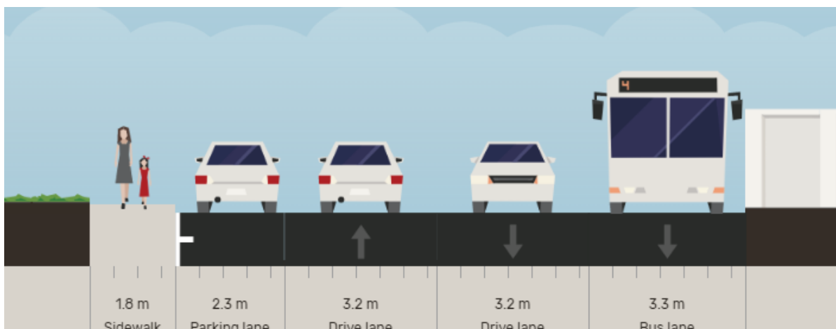
Figure 23: Chaytor St Segment 1 existing cross section
