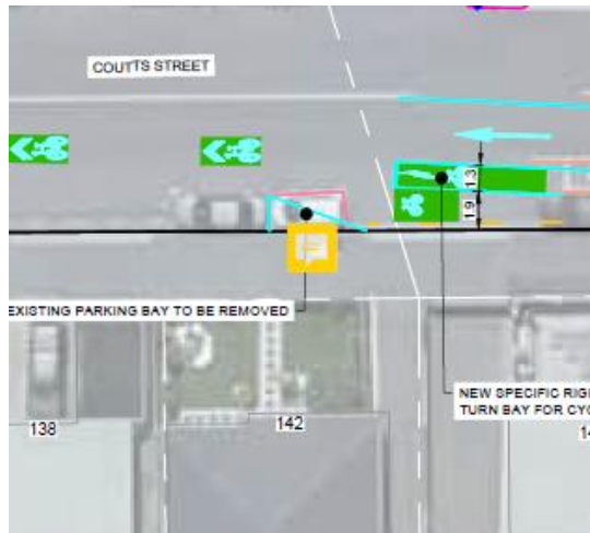
Figure 5-1: 142 Coutts Street parking removed
