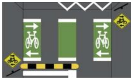
Figure 2-2: Driveway treatment solution
