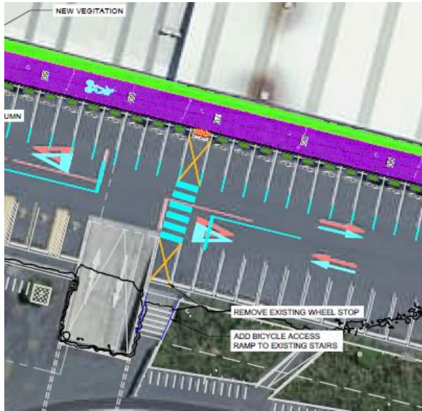
Figure 6-4: Crossing facility in car park
