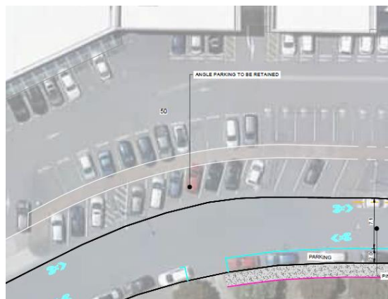
Figure 4-4: Angled parking being retained without buffer to the road
