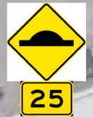
INSTALL "HUMP WN2" WITH "25 ADVISORY SPEED WG5" SIGN ON NEW METAL POLE
