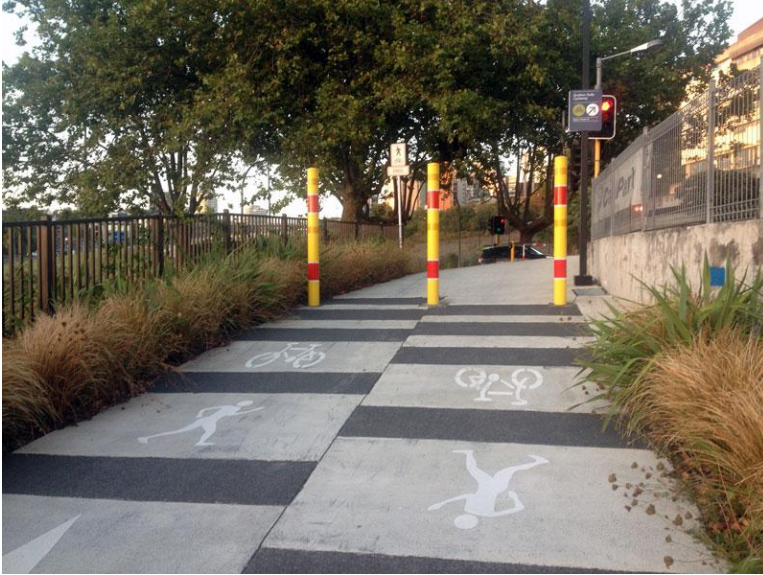
Figure 3.7: Example of pavement markings and textures on a shared path (Source: Waka Kotahi, Cycling Network Guidance)
