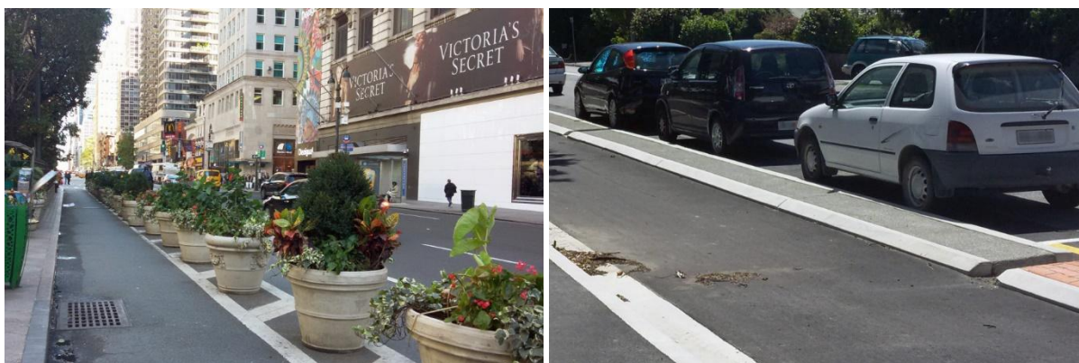
Figure 3.4: Example physical separators to provide protection (Source: Waka Kotahi, Cycling Network Guidance)
