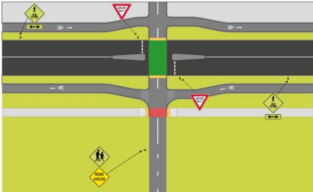
**Figure 15: Mid-block off-road bicycle path crossing. Adapted from Massachusetts Department of Transportation Separated Bike Lane Planning & Design Guide <sup>3</sup>.**
