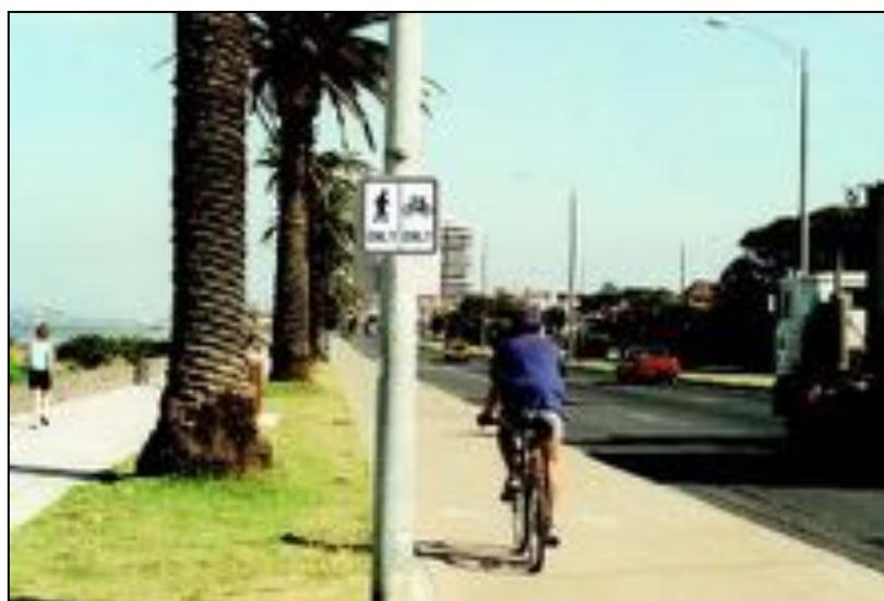
**Figure 8: Example of separated pedestrian and cyclist path**
